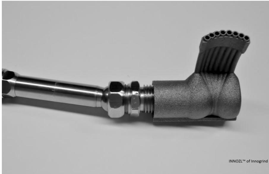
Optimized coolant conditions ID grinding, also for profiled grinding wheels
